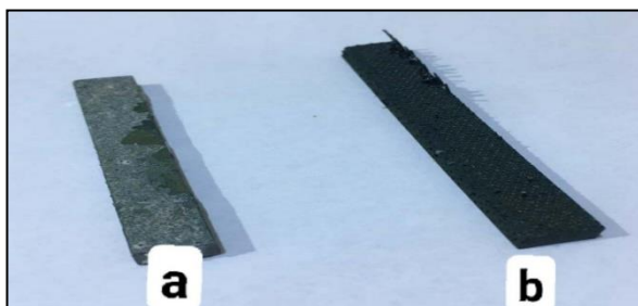
Fig.2 a) Investment casting sample (10X4X65 mm) b) Selective Laser Melting sample (10X4X80 mm)
