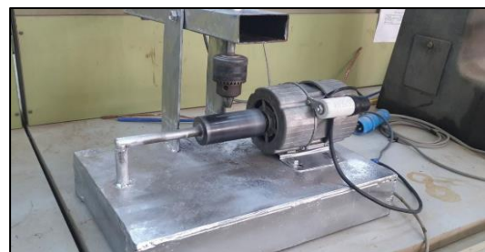
Fig. 4 Pin on Ring device of Wear Testing
